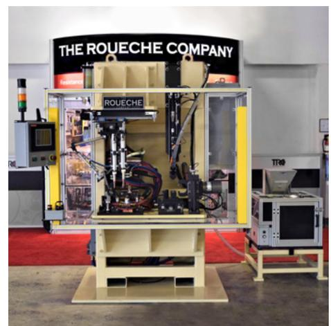
**TRC** can incorporate a variety of Integrated Fabricating Equipment into our custom resistance welders that can ultimately provide you with a turn key assembly while meeting the required cycle time and product requirements.
