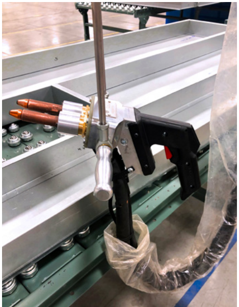
"C-Gun" Style Hanging Weld Gun System
